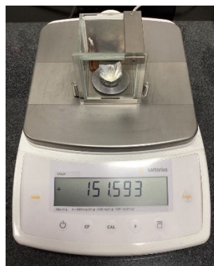
Weighing of 150 mg of milk in a DumaFoil
